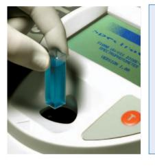
be made using standard 16mm diameter test tubes plus the cell holder may be removed for cleaning. Another version of the instrument, the WPA S1200T, is available with a factory fitted electrically heated cell holder for thermostatted measurements at 37°C.
